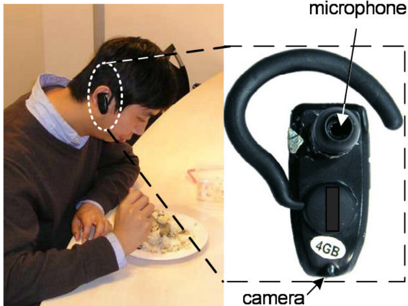
Left: a subject wearing the food-intake sensor during lunch. Right: the profile of the sensor.
