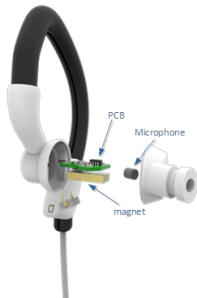
Figure: The ear-worn device with the microphone and PPG sensor.
